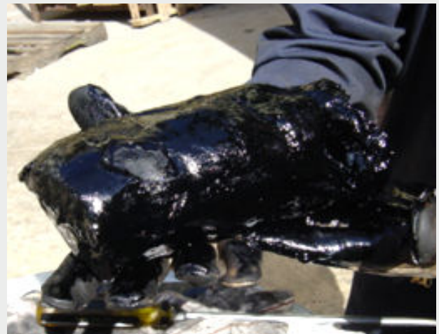
FIGURE 4: A CARBON LOG REMOVED FROM A HTS
